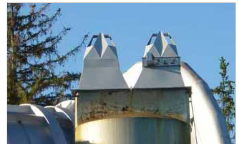
Illustration of the basic concept of the Advanced Dilution Nozzle Design
